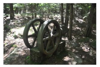
The air compressor used to drill holes in the granite
